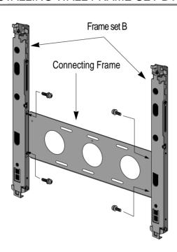
•Place frame set B on the left and right side of the unit and use the enclosed screws (M5) to secure them tightly.
